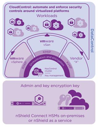
Entrust nShield hardware security modules (HSMs) secure the admin key and key encryption keys used to protect the Entrust KeyControl key management server.
